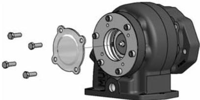
high-pressure rated grease or an anti-sieze grease. One-half ounce of grease added with a grease gun at periodic intervals should be adequate for maintaining this shaft. After greasing, re-place the cover over the shaft end.
