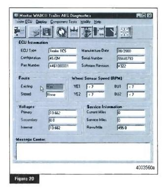
Check the Faults field on the Main Screen.
