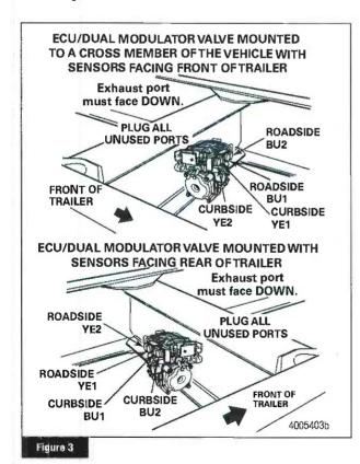
When mounting the ECU/dual modulator valve assembly to the trailer cross member, refer to SAE specification J447, Prevention of Corrosion of Motor Vehicle Body and Chassis Components. Follow all recommendations and procedures. Your supervisor should have a copy of this specification.
