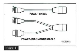
For industry-standard pigtail connector power cables, route the cable from the harness connector to the ECU/dual modulator valve assembly and secure it to prevent damage.
