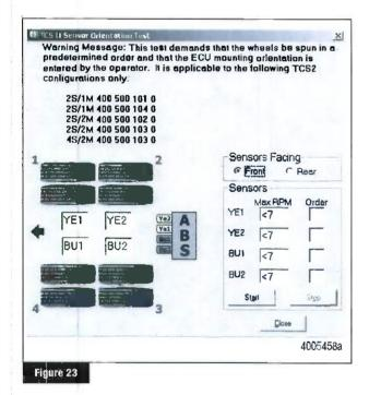
Click on *Front* or *Rear* in the *Sensors Facing* field to select the mounting orientation of the ECU/dual modulator valve assembly. Figure 24.
