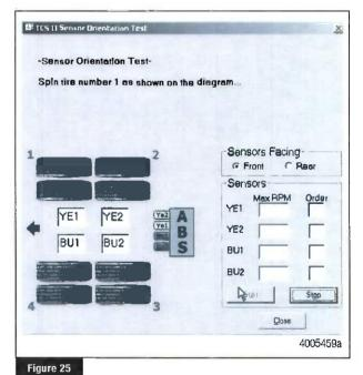
7. Follow the screen prompts, starting with 1, to rotate each sensed wheel end at a rate of 1/2 revolution per second. This rate equals a wheel speed of approximately 4 mph (7 kph). As each sensed wheel is rotated, check the color of the sensor identification block on the screen for results. Sensor identification boxes are located in the bottom left portion of the Sensor Orientation Test screen. Figure 24.
