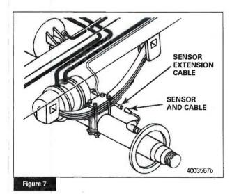
Route the sensor cable along the back side of the trailer axle to the ECU/dual modulator valve assembly. Route the cable with the brake hose. Do not overtighten the tie wraps on a cable. Overtightening can damage the cable. Do not tie wrap the molded sensor plug. The sensor extension cable must follow the brake hose to the ECU/dual modulator valve assembly to allow for axle jounce and rebound.
