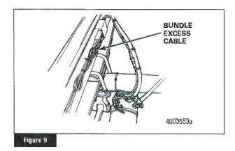
Secure excess cable in the sub-frame of the vehicle or along the air hoses as appropriate. Excess cable should not exceed two feet (0.61 meter).
